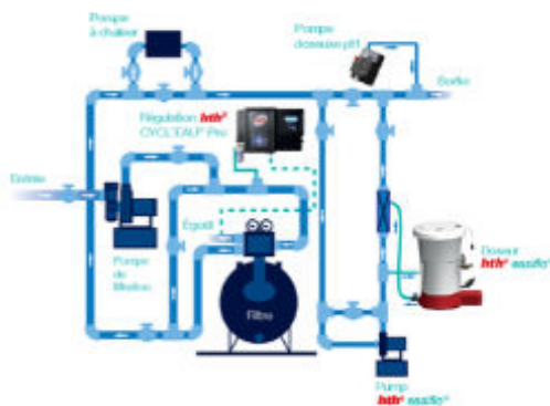
Typical installation diagram for an hth CYCL'EAU ® Pro control system with hth easiFlo ® feeder
